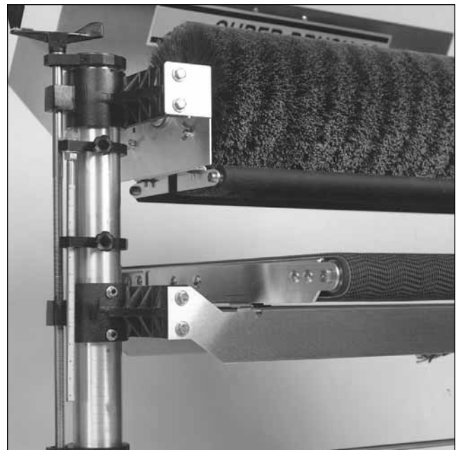
Fig. 16. Height controls on outboard side.
