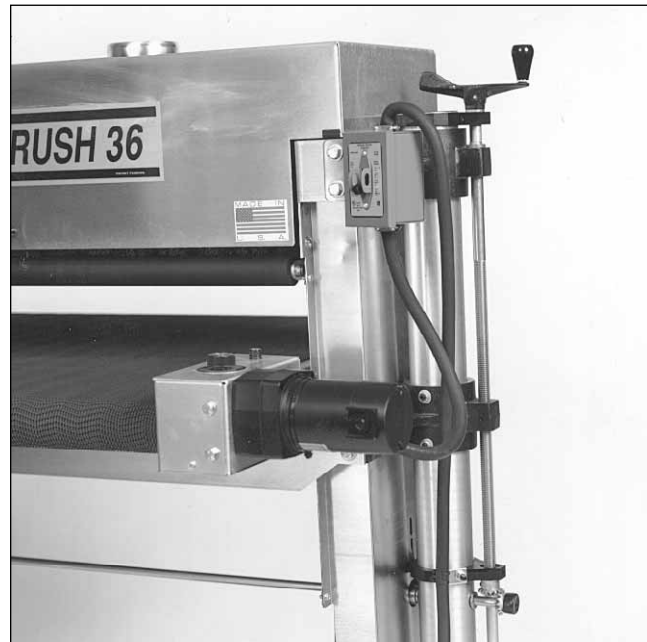
Fig. 26. Conveyor motor control box and brush on/off switch.
