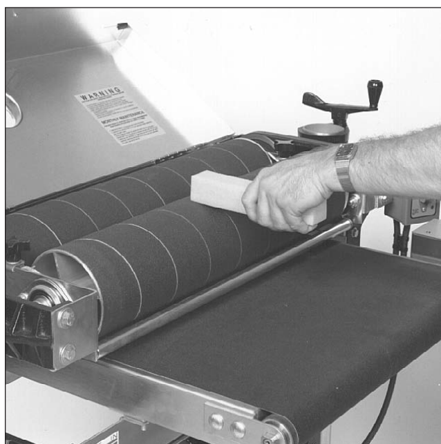
Fig. 18. Cleaning abrasive strips.
