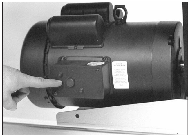
Fig. 4. Thermal-overload switch, on some models.
