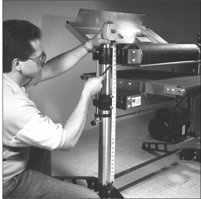
Fig. 24. Comparing drum support casting heights.
