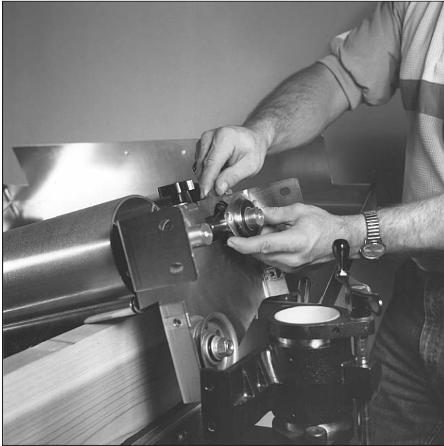
Fig. 43. Removing rear bearing (inboard side).
