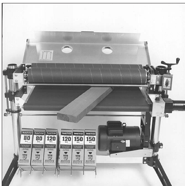
Fig. 17. Offset stock feeding angle.
