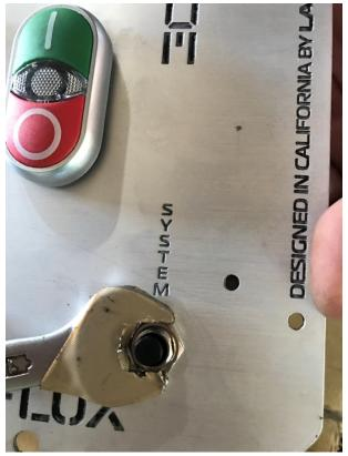
9. Replace with the 15A overload protector and close the control panel and bolt on to the stand to complete the setup for 220V.
