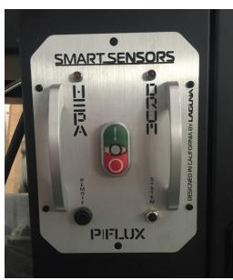
2. Remove the Control panel from the panel to get into the box behind.
