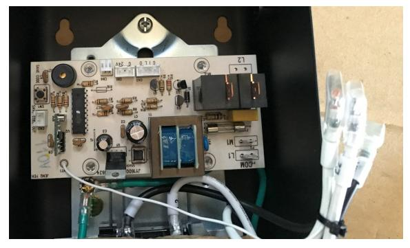
5. Carefully and gently loosen the four plastic bolts on the circuit board and set aside for use in the next step. Remove the 110v circuit board and replace with the 220v circuit board. Make sure the direction of the 220V circuit board is attached in the same position as the photo shown below.
