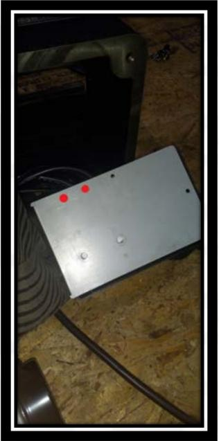
Remove the center black, red, and white wired connector from the control board. Then remove the black and white connectors from the control board.
