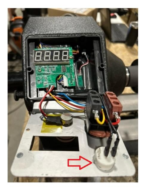
You will need to push on the 2 sides to remove the switch from the panel. You may need to use some pilers to remove. After the wires and switch are removed
