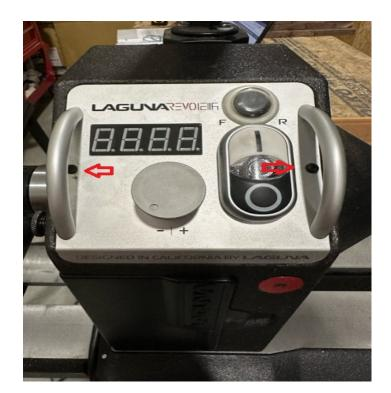
After removing the control panel, you can open it up and remove the screws located on the DRO.
