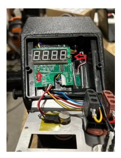
Once you remove the screws flip over the DRO and remove the wires for the switch.
