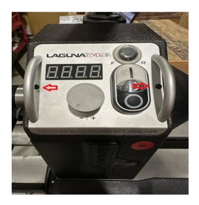
After removing the control panel, you can open it up and remove the screws located on the DRO.
