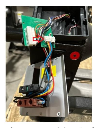
Once you have removed the wire from the DRO you can remove the switch from the control panel.
