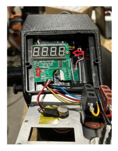
Once you remove the screws flip over the DRO and remove the wires for the on/off switch. These are the red, blue, and yellow wires.
