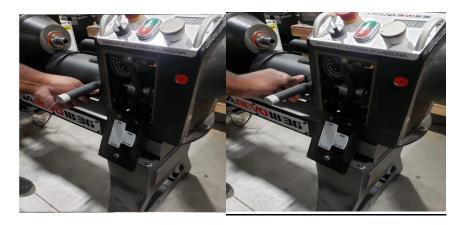
**3.** Lift up on motor adjustment handle to lift motor up to physically lift motor into a position where the belt will loosen.
